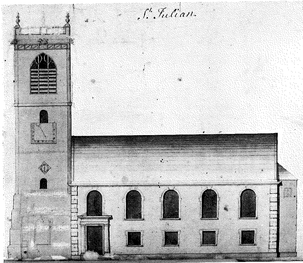
PLATE 2 ST JULIAN'S, SHREWSBURY, 1749–50, DESIGNED BY THOMAS FARNOLLS PRITCHARD. THE ARCHITECT'S PRESENTATION DRAWING OF THE SOUTH ELEVATION, SHOWING THE RETAINED MEDIEVAL WEST TOWER (SRR: 6001/299).
